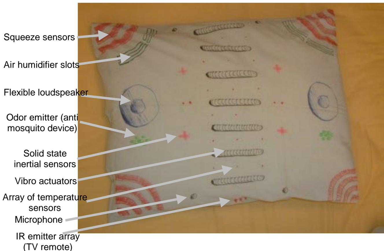
Although there must be many electronic elements in the pillow, it has to be completely soft and flexible. To power the internal electronics, sensors, and actuators, the pillow has built-in thin film lithium batteries that are charged with induction from the mattress (no direct conducting contact necessary, works through bed sheets and pillow cover).
