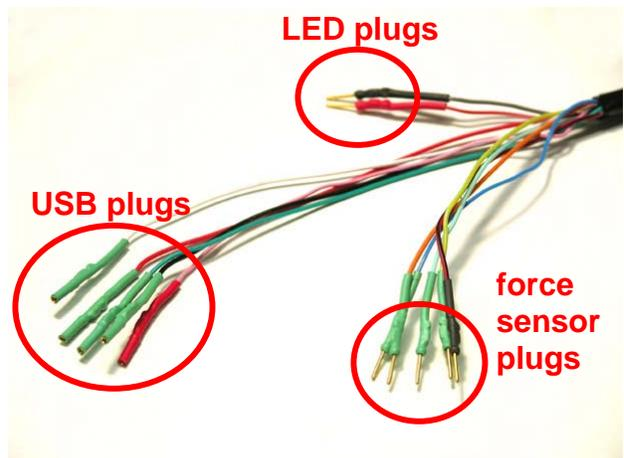
Once the ends of the cable are connected to the board, the wires should be taped down to the box so that they will not be accidentally unplugged!
