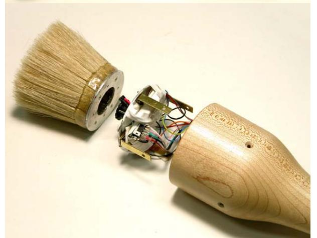
Finally, please follow the color code of the shrink-wrap when connecting the ends of the wire.
