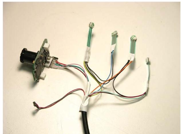
The force sensors must be secured on the inner aluminum ring without being bent. If the sensor's film-strip is bent or is moving around, it interferes with the sensor reading.
