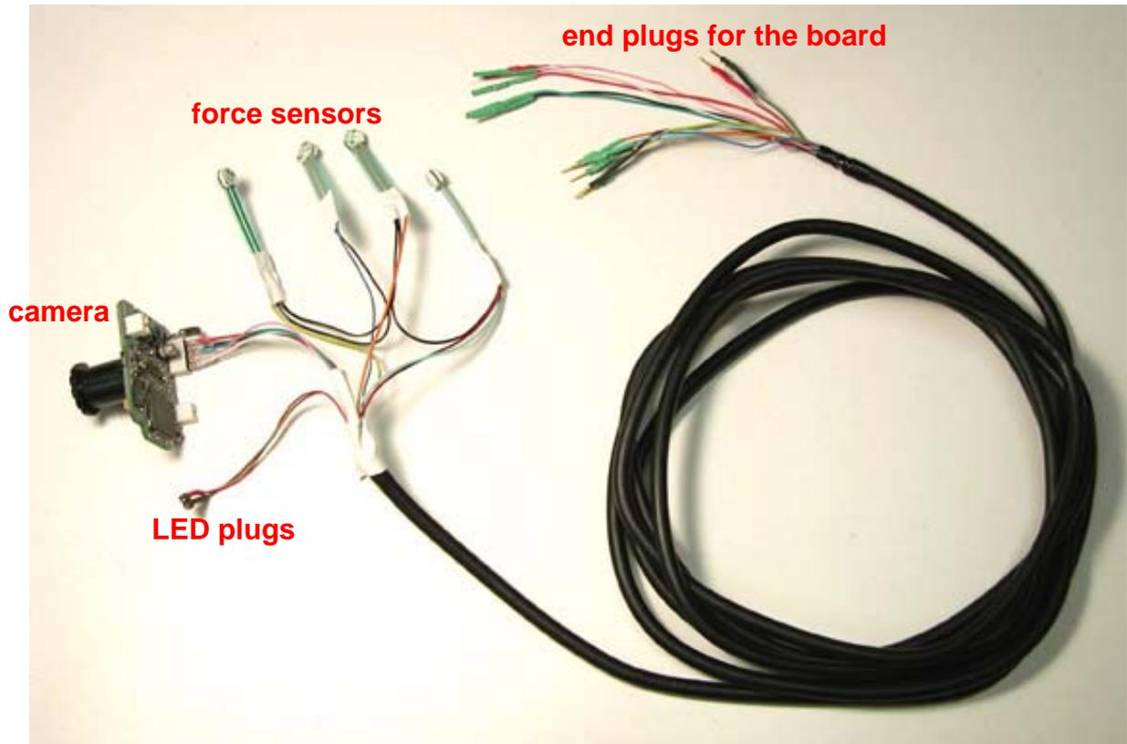
The **camera**, **LED plugs**, and **force sensors** must be neatly encased inside of the brush (see the pictures below).
