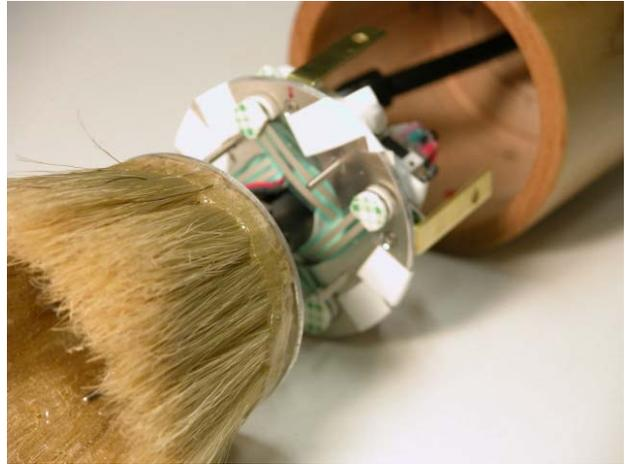
The force sensors are attached to the surface of the inner ring with a strong double-sided tape. Even though both sides of the sensors have double-sided tape, one side is for the “cushioning” purpose only. In other words, do not peel off the stickers on the outer side. The sensors should be only attached to one side (the inner ring).
