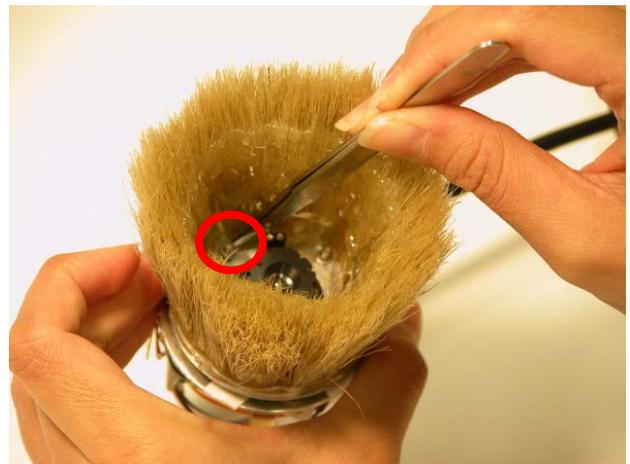
Once you remove the nuts from the bolts, you can remove the bristles/hair ring from the inner ring.
