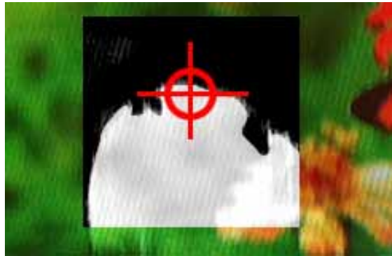
Figure 6. Blob detection and fingertip determination from the hand image within the pressed key region
