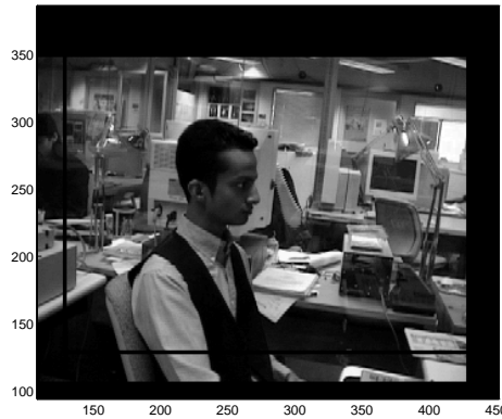
Figure 12: Estimated alignment of frames. The box shows where frame 2 lies in relation to frame 1.
