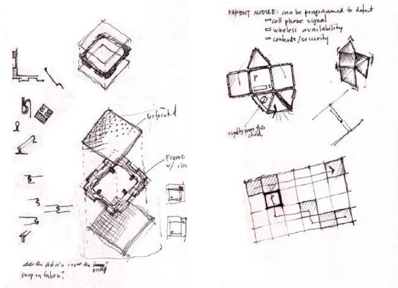
Simple geometries of squares and triangles were chosen because they are easily recognizable and can be effortlessly manipulated into two and three-dimensional shapes. Additionally, the dimensions were chosen to fit comfortably when grasped by the human hand. Next, modular shape choice and its influence on an object's degree of configurability were investigated.
