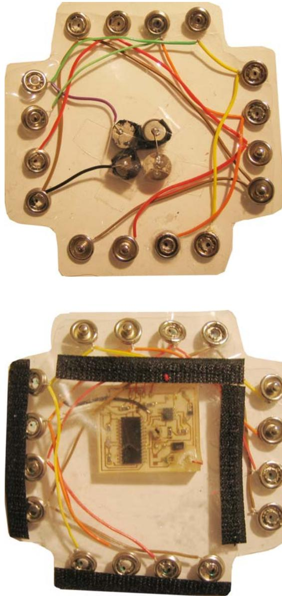
Tangible study revealed that the snaps were ultimately disappointing because their aggregate weight compromised the feel of any object that was constructed out of such a configuration.
