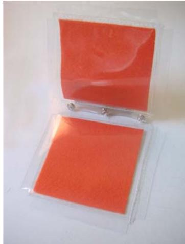
It was decided early on (for reasons that will be explained later) that the communication bus would be a four-channel protocol that transmits power, ground, data, and clock through the conductive snaps. A diagram indicating how the printed circuit board (PCB) could be wired to the snaps was mocked up and construction on the blocks began.
