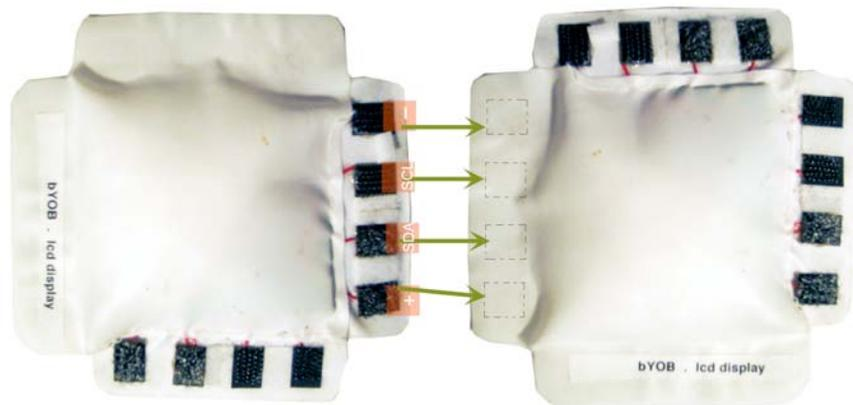
As stated before, corresponding pads on each edge are connected together via internal wiring so the ground pad on one edge is connected to all of the corresponding ground pads on each subsequent edge- and so on for each type of pad.
