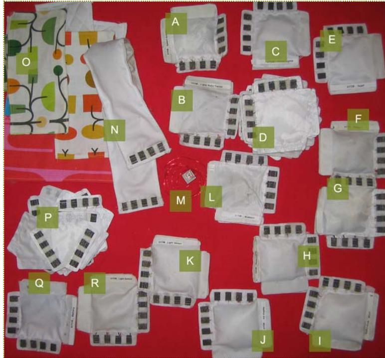
**[K,R]** Light sensor blocks repeatedly monitor the ambient light level using a photocell. These blocks will ask connected illumination blocks to light up the object they are a part of (e.g. the bottom of a purse) when it gets dark.
