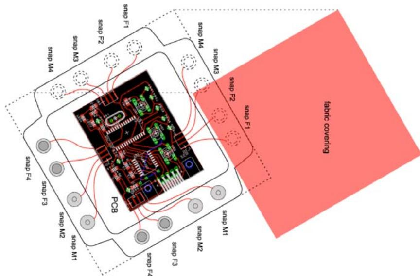
Clear vinyl was chosen for the outer shells because it is durable but also because it allowed an exploration into a new aesthetic. The four edges of snaps were affixed to each side.
