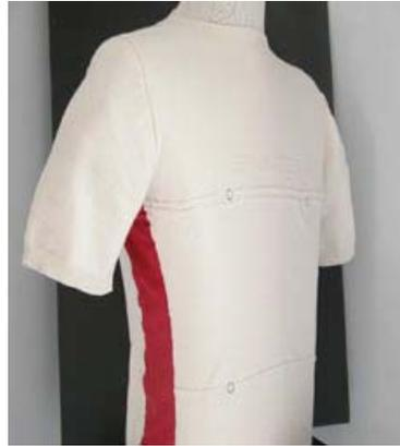
The Sensatex smart shirt collects biometric data with woven and knitted conductive fibers and sensors. Sensatex researches how their proprietary system can be integrated into many types of fabric without affecting the integrity of the material [Sensatex, 05].
