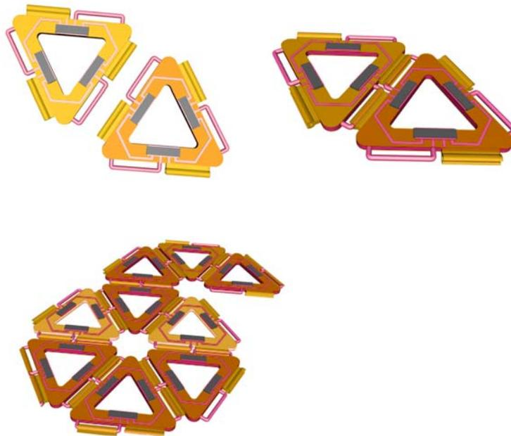
Printing this connector technology out on the FDM (fused deposition modeling) machine revealed that neighboring connections were loose. Moreover, because a separate channel for electrical conduction would have to be added into the design, the method proved too complex to pursue any further.
