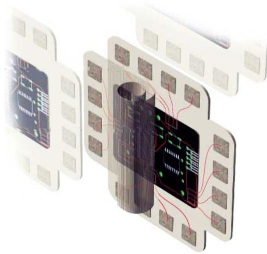
In order to connect soft items like hook and loop to hard epoxidized electronics boxes, we tested many types of thin, durable wiring that could be held by conductive epoxy after drying overnight. No electronics and wiring are visible to the user in this configuration.
