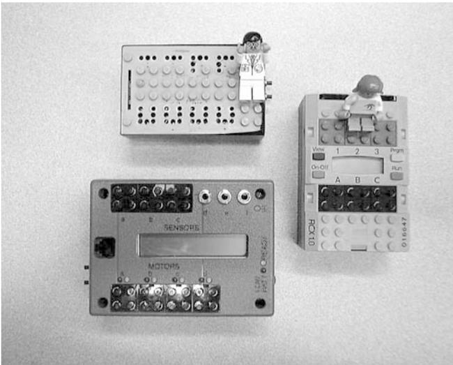
**Fig. 4** The evolution of programmable bricks: early *Gray Brick* (top); later *Red Brick* (bottom); and commercial LEGO RCX (right) aka *Yellow Brick* (Photo by F. Martin)
