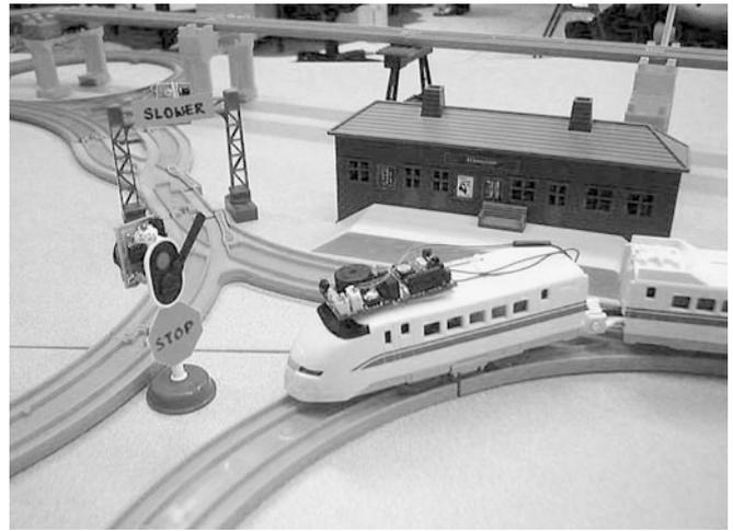
Fig. 9 Tomica train set augmented with a Cricket that heeds IR beacon signs (prototype). Tomica is a trademark of TOMY Company, Ltd
