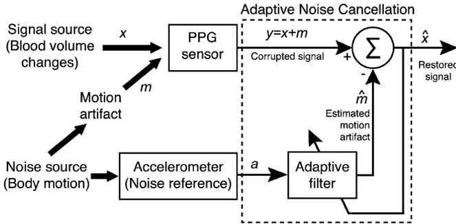
Fig. 3. Block diagram of ANC configuration.
