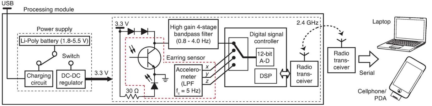
Fig. 2. Overview of the integrated system architecture.
