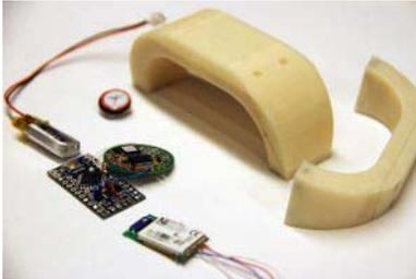
**Figure 6.** Electronic components and 3D printed bracelet.
