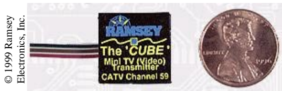
Figure 17: Example for very light video transmitter (Ramsey C2000, weight 2.8 grams)
