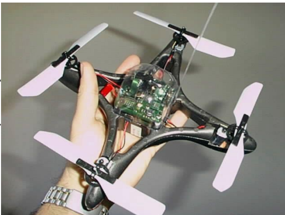
Figure 7: GyroSaucer by Keyence (weight 143 grams, diameter about 26 cm)
