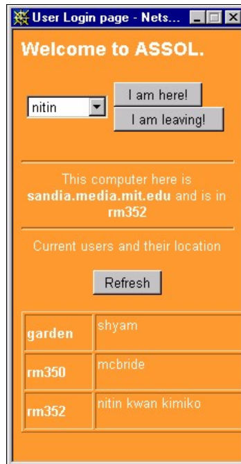
Fig. 7. Login window. The user can tell the ASSOL where she currently is. The window also shows in which room this computer is located, as well as who is currently in which room
