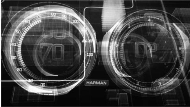
Figure 2. Example of a transparent instrument cluster (this illustration is in 2D, the actual system renders in 3D).
