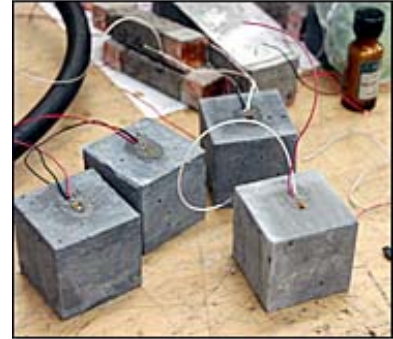
Kevin Rivoli for The New York Times Dr. Deborah Chung of the State University at Buffalo, above, with smart concrete. The concrete, being tested, left, blocks radio waves.
