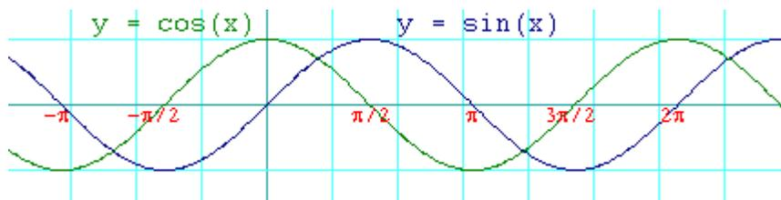
*The two analog output signals that combined give the heading of the sensor.*
