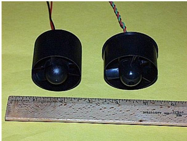
*New EDF 200 (left) compared to old Cox/Estes. It is even smaller in diameter, but uses the same motor with a different nominal voltage..*
