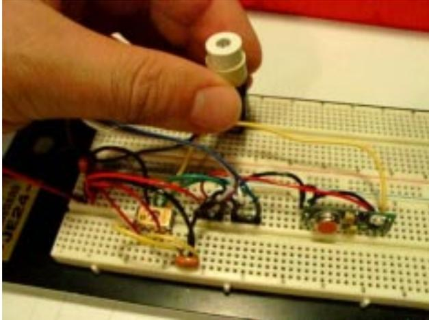
*On the lower left side is the PIC visible (UV erasable), on the right side the Radiometrix transmitter. I am holding the compass. This configuration was for debugging; eventually, all components will be replaced by surface mount equivalents and soldered directly to each other.*
