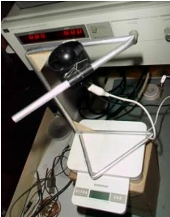
*Thrust measurements: The ducted fans were mounted on a bent aluminum tube that is reinforced with plywood at the corners. The whole construction was taped onto the Soehnle scales that can measure the thrust with an accuracy of 0.1 grams. The HP power supply can deliver 0-20V, 0-120A, max 1000W.*
