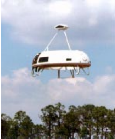
Figure 8: Cypher by Sikorsky (diameter 186 cm, weight around 120 kg).
