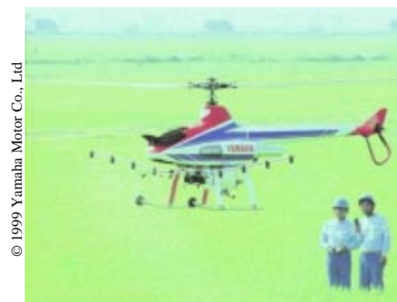
Figure 18: A Yamaha R-50 helicopter, overall length 3.57 meters, as used by M. Sugeno for his voice controlled helicopter interface.
