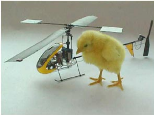
Figure 6: Pixel 2000 made by Alexander van de Rostyne (weight 48.2 grams, length about 30 cm).
