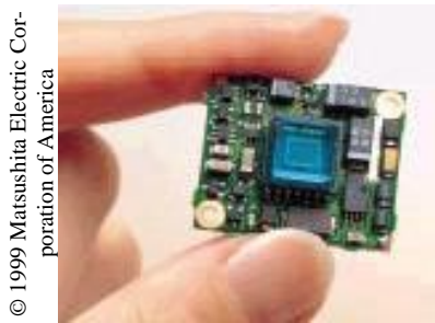
Figure 16: Another very light CCD board video camera (Panasonic GP-CX161P, weight 8 grams)
