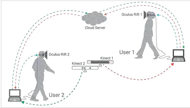
**Figure 2. MetaSpace system configuration.** Each user wears an Oculus Rift virtual reality head mounted display and can see themselves (first person view) and the other user's avatar on their screen. Each user is fully tracked with a Kinect and body movements like walking, waving etc of each user are transmitted through the cloud server such that everyone can see everyone and feel their presence in the virtual world similar to that in the real world.
