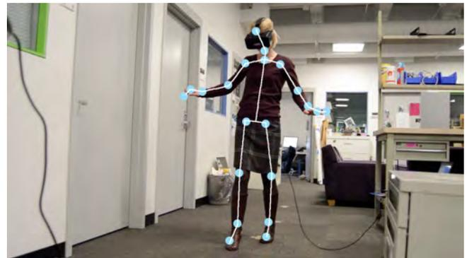
**Figure 4. User 1 walking down the hallway (real) and bridge (virtual) toward User 2 (Figure 3) waving at them. User 1's skeleton is tracked by the Kinect and their physical movements are mapped to their avatar's movements.**
