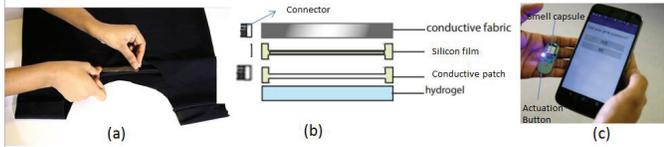
**Figure 4.** (a) stick-on sensor with hydrogel adhesive patch, (b) schematic diagram of the stick-on sensor, (c) communication module and the companion mobile application that connects to the sensor and calls for help as needed.
