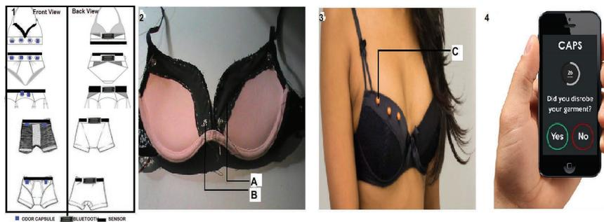
**Figure 1.** From left to right: a) Graphic shows how our sensor is attached to clothing. b) The stick-on sensor is made of stretch-sensing fabric A, in black, and clipped on to existing underwear B. c) User wearing our smart clothing. The design is comfortable and unobtrusive. The three dots visible on the bra labeled C are the odor capsules. d) The companion mobile application that connects to our sensor through a communication module and calls for help as needed.
