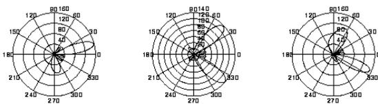
Figure 4: Directivity Pattern of Broadside Array with Cardioid Elements steered at 15, 45, and 75 degrees. Note that the reference point of the broadside array geometry (Figure 3) should be aligned with the center of each polar plot
