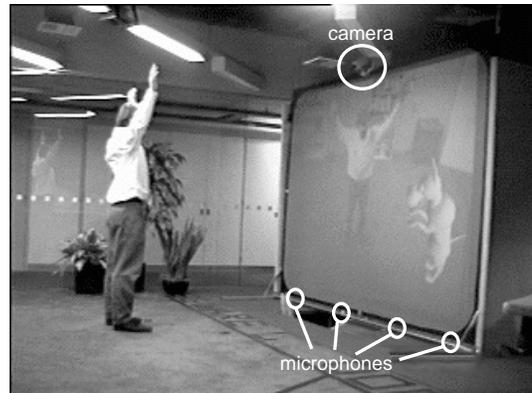
Figure 1: Location of the camera and microphone array in the virtual environment
