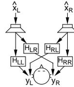
Figure 6: Transfer functions from speakers to ears in stereo arrangement.
