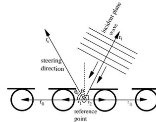
Figure 3: Broadside Microphone Array Geometry and Notation
