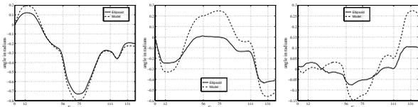
Figure 8: Head-tracking results for calibrated sequence: plots shown are for the alpha, beta, and gamma parameters (rotations around the z,y, and x axes, respectively).
