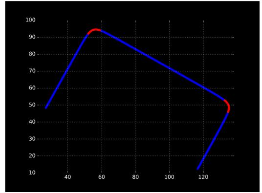
(a) The result of dividing a single sub-path into separate segments. The clustering algorithm used here sets segment boundaries before and after curves. The sub-path segments in red indicate areas where the longitudinal speed required to adhere to lateral acceleration limits is below the legal speed limit of 11.1 m/s (25 mi/hr).
