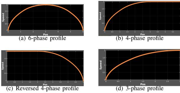
Fig. 10. 6, 4, Reversed 4 and 3-phase profiles, displayed as speed vs. position along path.
