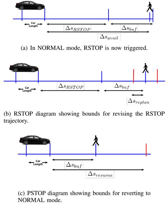
Fig. 6. Graphical representation of static and dynamic thresholds used to trigger state transitions.
