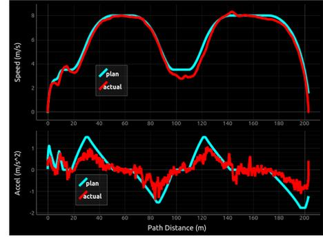
Fig. 12. Planned speed and longitudinal acceleration vs. measured values
