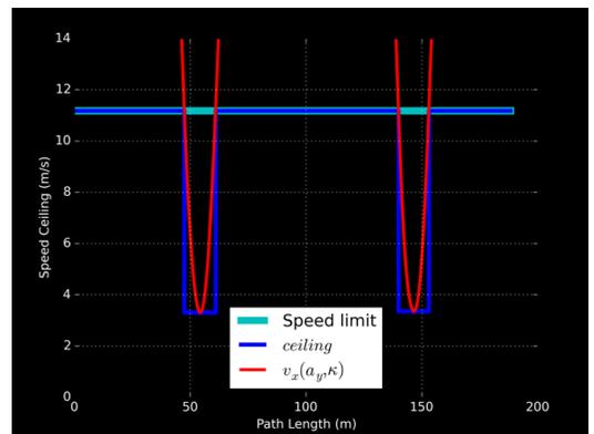
(b) An example of how the sub-path's segment boundaries are determined, as well as how  $v_m$  is consolidated to determine the speed ceiling for each segment. The x-axis corresponds to distance along the subpath above. The legal speed limit of 11.1 m/s (25 mi/hr) is shown in cyan. The longitudinal speed required to adhere to lateral acceleration limits is shown in red. The resultant speed ceiling ( $v_m$ ) is shown in blue.
