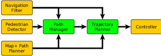
Fig. 2. Primary system components. The *Path Manager* and *Trajectory Planner* components (in green) are presented herein.
