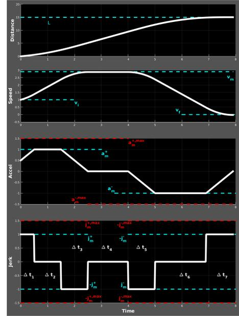
Fig. 9. 7-phase constant jerk profile along the curvilinear distance axis. All values needed to completely parameterize a single path segment for trajectory are labeled here.
