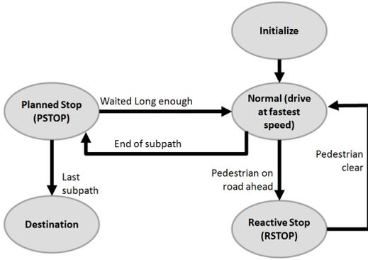
Fig. 4. State Transition Diagram for Path Manager. System transitions from NORMAL to PSTOP mode at each stop sign. In the presence of a pedestrian the system transitions to RSTOP.
