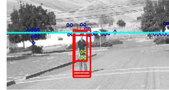
Fig. 3. Showing detected pedestrian by the computer vision system
