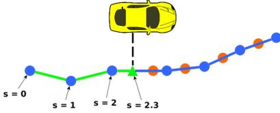
Fig. 11. Showing projection of the current position of the car shown by green triangle to  $s$  coordinate system. Each circle represents a node, and the lines between them are links. The orange dots indicate future trajectory samples which are sent to the controller.
