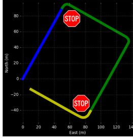
Fig. 5. Dividing the path into sub-paths at stop signs. The Trajectory Planner is serially called for each sub-path shown in different color.
