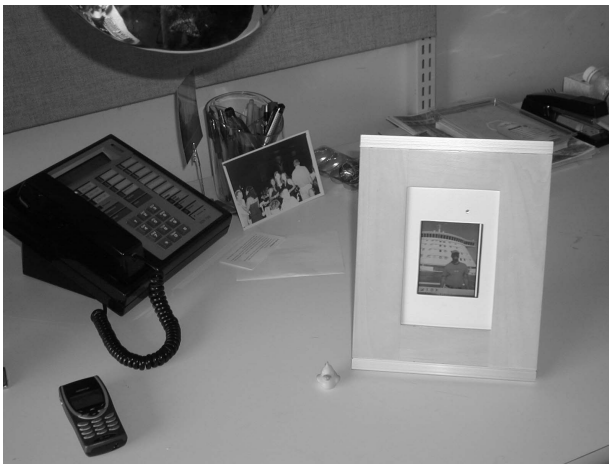
Figure 1. The TalkBack Answering Machine (picture frame on the right).
