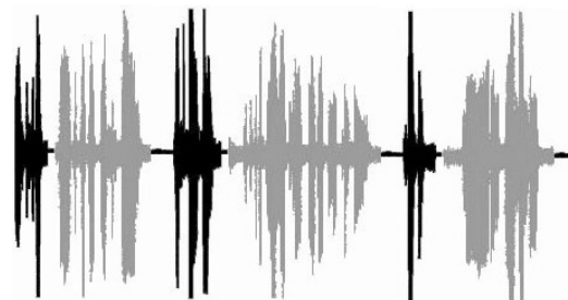
Figure 2. Waveform of message sent back to caller using TalkBack. Each response, seen in grey, is interspersed with a few seconds of the original message time compressed, seen in black.
