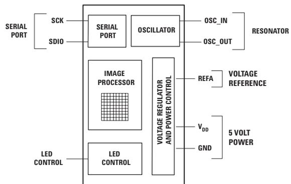
Figure 6. Block diagram of ADNS-2620 optical mouse sensor.
