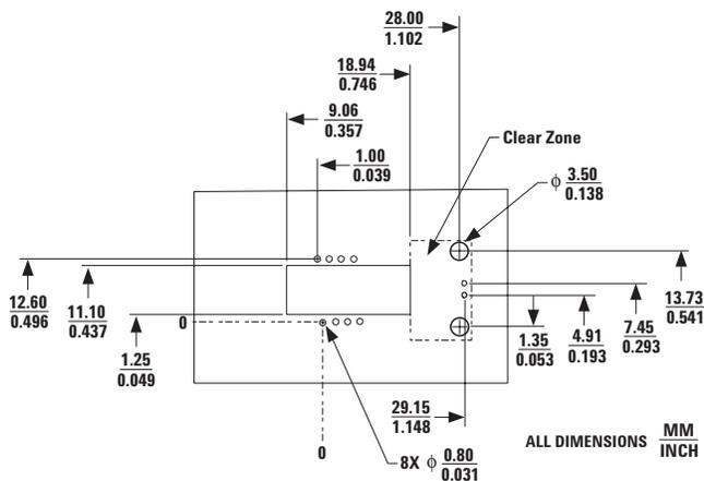
Figure 3. Recommended PCB mechanical cutouts and spacing.
