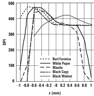
Figure 14. Typical Resolution vs. Z (comparative surfaces)
