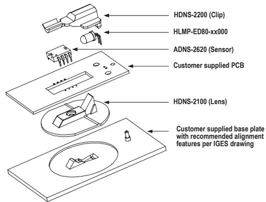
Figure 5. Exploded view drawing.
