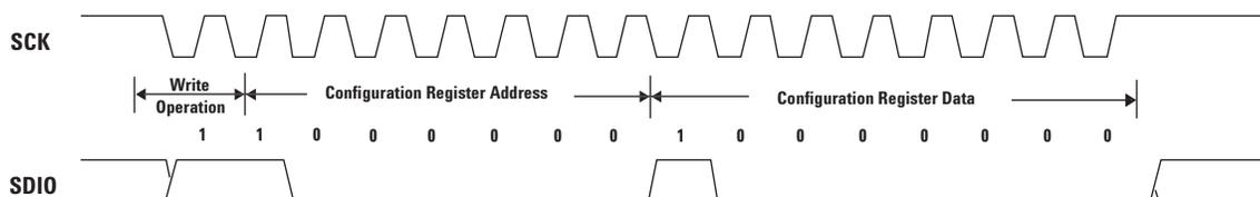
Figure 31. Soft reset configuration register writing operation.
