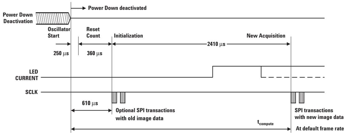
Figure 11. Details of wake-up timing after PD.
