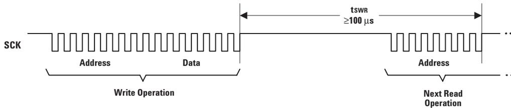
Figure 26. Timing between write and read commands.
