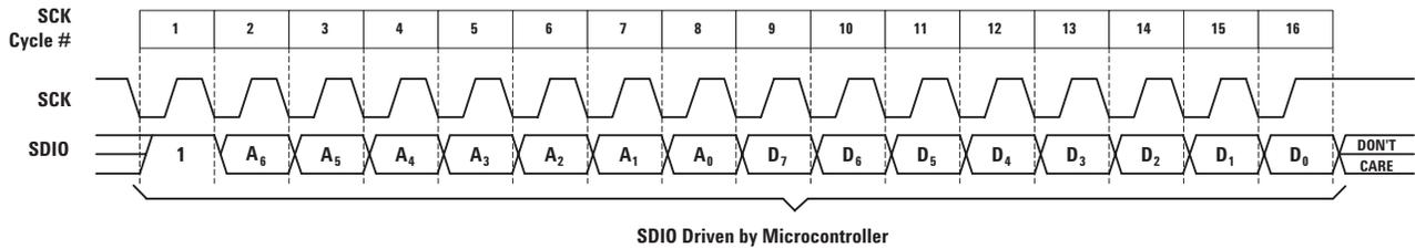
Figure 19. Write operation.
