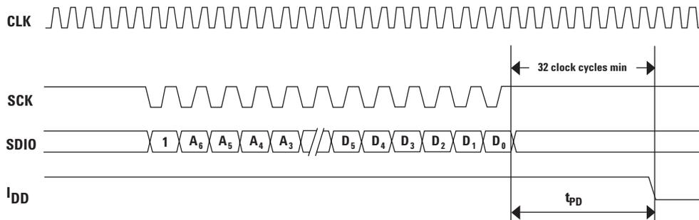
Figure 12. Power-down timing.
