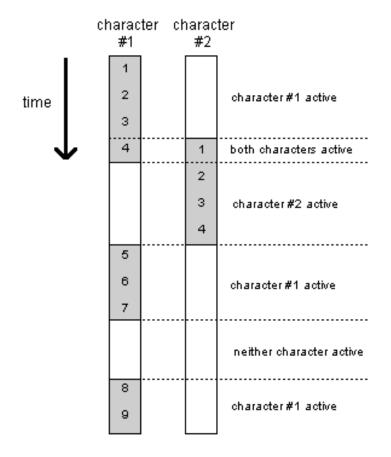
Figure 30: Unsynchronized approach to the multithreaded narrative model. The vertical columns represent the two character threads, the numbering indicates the narrative segments, and the shaded areas show when each character is active. In this example, character #2 is activated at a later time than character #1. This means that by the time character #1 has already reached narrative segment 4, character #2 will be starting its monologue at narrative segment 1.
