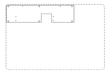
Figure 52: Corel Draw design of the circuit board support layer. The dotted line indicates the edge of the top four layers.
