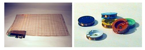
Figure 36: The tag-reading surface consists of eight antenna loops arranged in a flat plastic cover (left). The tags consist of a wire wrapped around the outside of a small plastic holder, in parallel with a capacitor concealed inside the holder (right).
