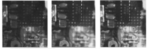
Fig. 9. Multifocus composite image. The original images with limited depth of field are shown in (a) and (b). These are combined digitally to give the image with an extended depth of field in (c).
