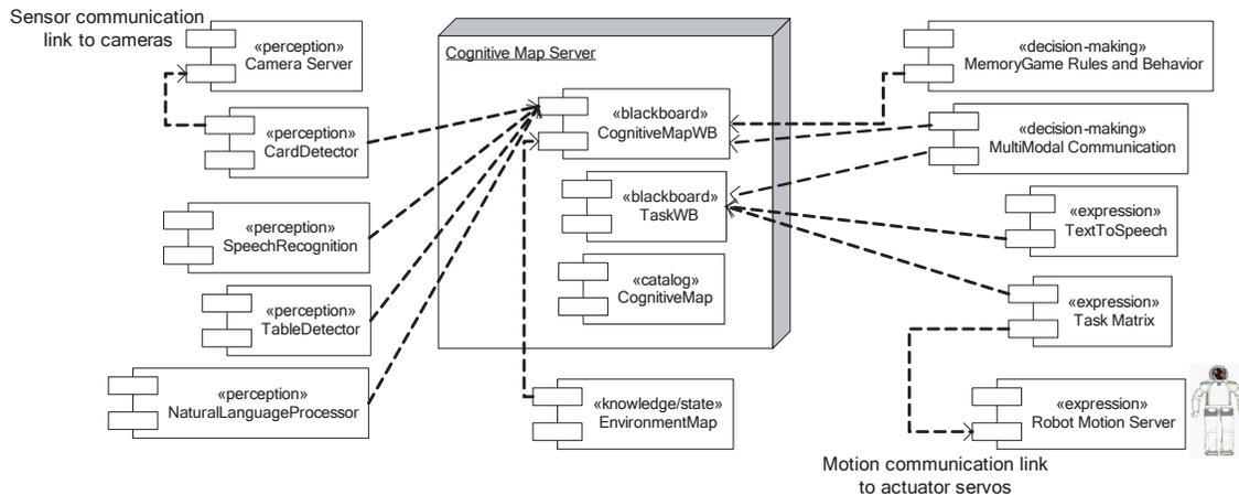
Fig. 2. Overview of the Cognitive Map robot architecture: Representative components depicted showing connectivity to the central Cognitive Map server. Component types are labeled above name. Arrow directions depict dependencies on various interfaces (not message directions).
