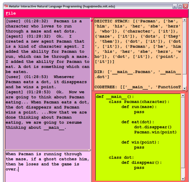
Figure 1. A screenshot of Metafor. Clockwise from the lower left corner, the four windows display 1) the narrative being entered; 2) an interaction log; 3) Metafor's representation of the parse tree (for demo and debugging purposes only: not shown to beginning users); and 4) the visualization code, in Python.
