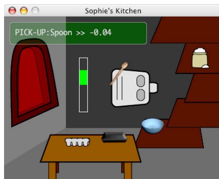
Fig. 1. Sophie’s Kitchen . The robot is facing the shelf, holding the spoon. The vertical green bar is controlled by the human and here shows a positive interactive reward of circa +6 .
