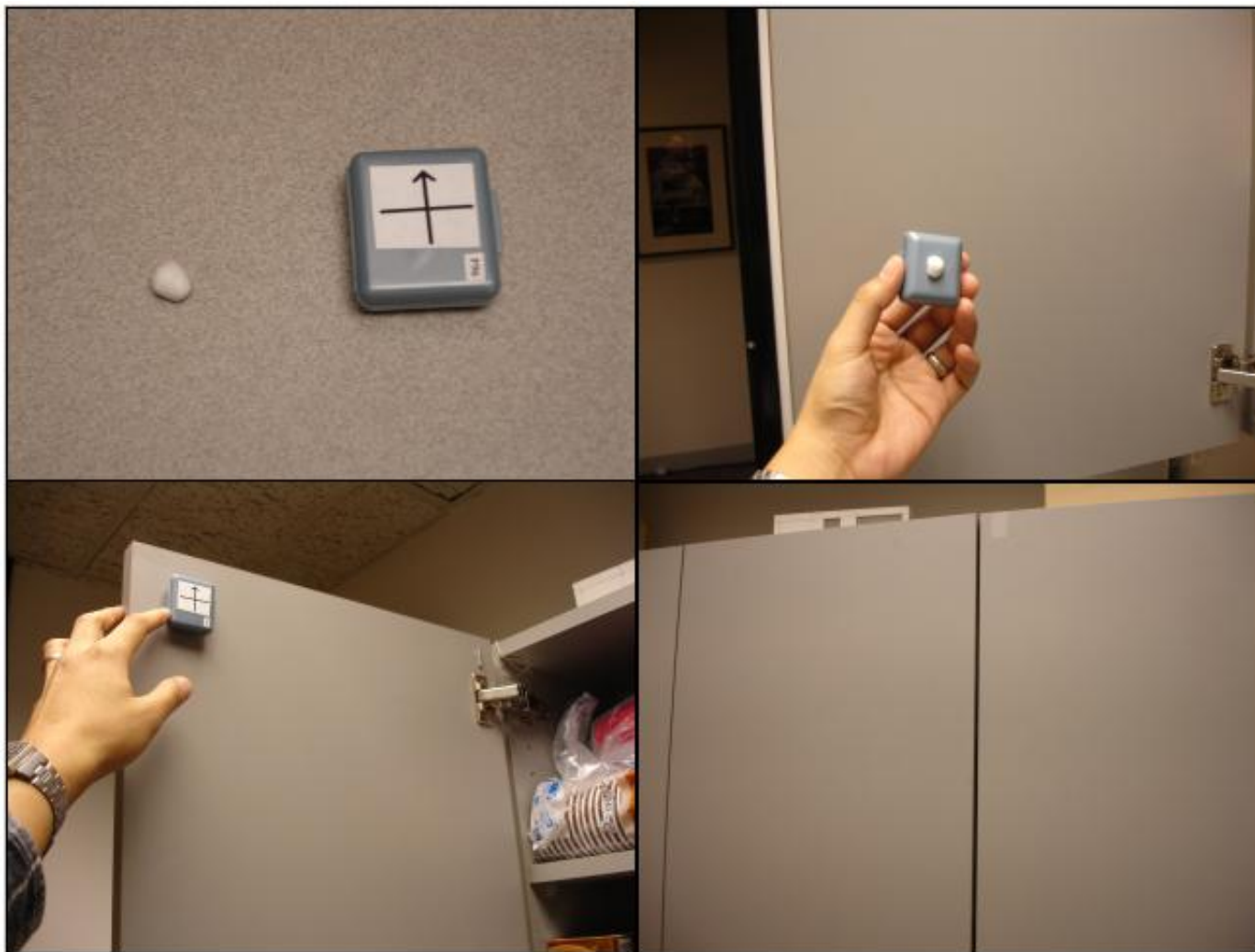
Installation procedure for stick-on MITes
