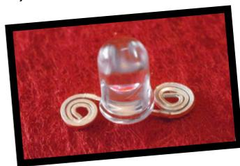
Red and black permanent markers can be used to color-code the positive and negative legs of each LED.
