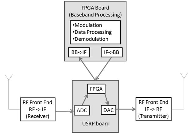
Fig. 3. Block diagram showing the design of the board [5].
