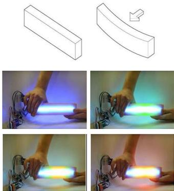
**Figure 2:** Color mapping of the beam in bending. The areas with greatest stress are shown in red and minimal stress in blue. Note that the center of the beam gradually changes color from blue to red as the force increases.
