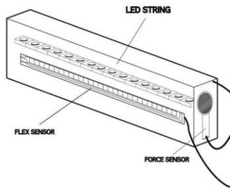
**Figure 4:** The beam block contains a flex sensor, two force sensors and a LED strip.
