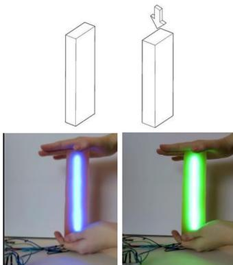
**Figure 3:** Color mapping of stress in the beam during axial loading.
