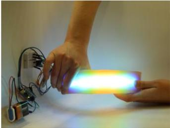
**Figure 1:** We prototyped a simple beam that visualizes axial and bending stress on the physical beam itself.
