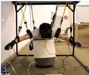
**Figure 1.** Amphibian is an immersive virtual reality system that enables people to experience ocean SCUBA diving in a convenient terrestrial setting. Images above show (a) the Prototype II suspension frame and (b) a user suspended in the harness, as needed for experiencing Amphibian.
