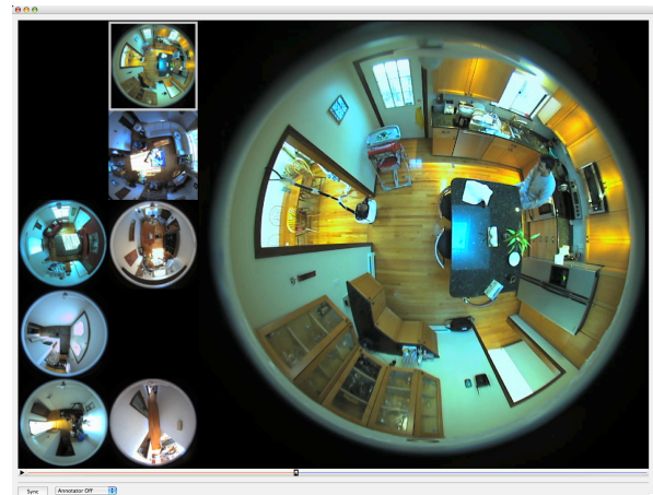
Figure 3: The TotalRecall video player, displaying low resolution video clips of all active channels on the left, and a single full resolution clip of the selected channel on the right.
