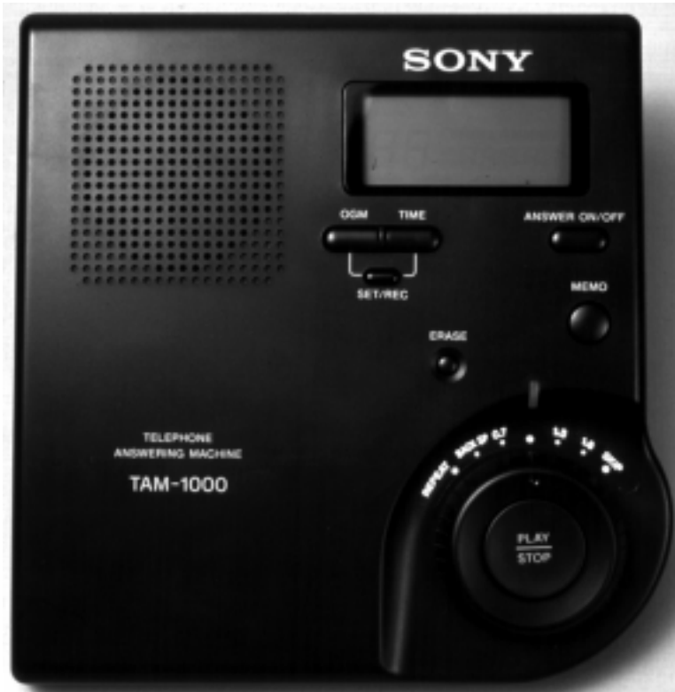
Fig. 1-1. A consumer answering machine with time compression.
