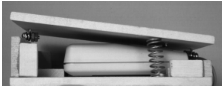
Fig. 2-2. Side view of the “footmouse.” Note the small screws used to depress the mouse buttons.
