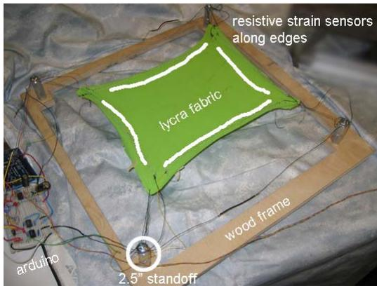
Figure 2. System design of hardware and mechanical setup
