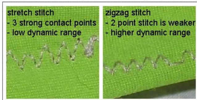
Figure 3. Stretch stitch (at left) is stronger and exhibits lower dynamic range than the zigzag stitch( at right)
