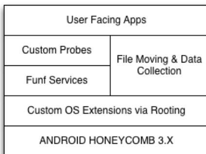
**Figure 3. Tablet architecture**
