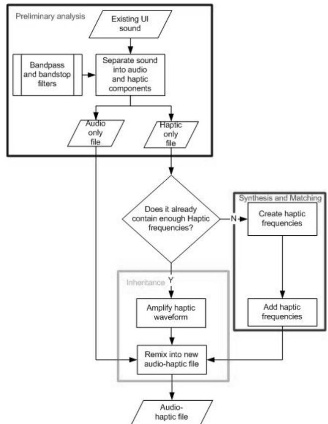
Figure 8 – Flowchart showing the method and path of design for the Inheritance and Synthesis/Matching techniques
