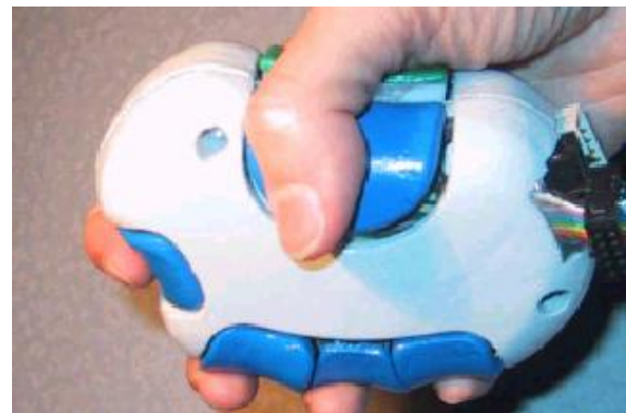
Figure 12. Problem with grip. The user may inadvertently squeeze the buttons while simply holding the phone.
