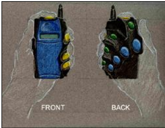
Figure 8. ComTouch adds a tactile communication channel on top of a cellular phone.
