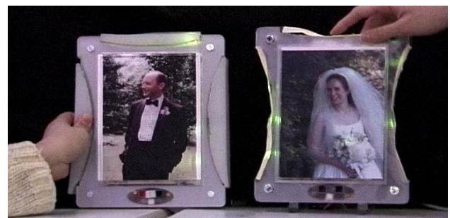
Figure 7. Sensory mapping embodiment for LumiTouch. Then the left user presses, it lights up the other frame. The top left area gives feedback of the color pressed.
