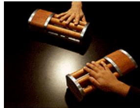
**Figure 1. InTouch allows rolling to be shared**
