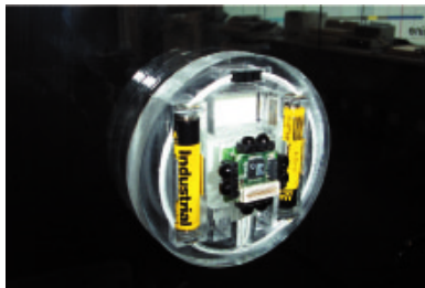
(a) 4-IR Pushpin without speaker. The four IR transceivers provide directional communication only along the horizontal and vertical axis.
