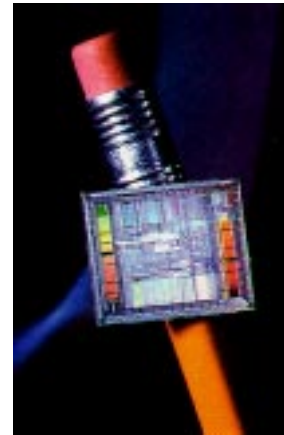
FIGURE 11-4. The Alpha 21064 chip from Digital Equipment Corporation measures 1.39 x 1.68 cm in size (this picture shows it roughly two times the actual size) and contains 1.68 million transistors. This is the chip that runs most of Ymir.
