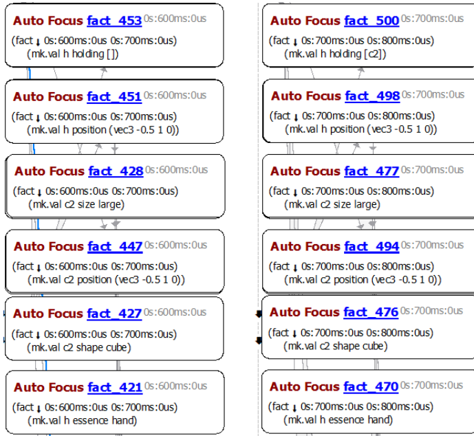
Figure 7.6: The facts in the right column are the observations that come after those in the left column. The positions of h and c2 are vec3 properties that represent the 3D positions of all objects in the Webots simulation environment. The size, shape, and essence are the other defined properties for the entities, h and c2 that have ontological symbolic values.
